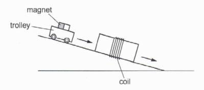
An electromotive force (e.m.f.) is induced in the coil. A graph of the e.m.f. against time is plotted.
