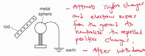
The earth connection is removed and then the rod is removed.
